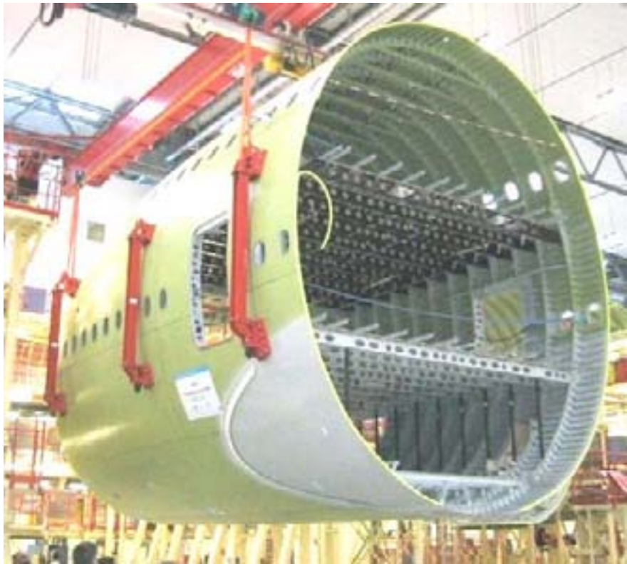
CFRP floor beams
