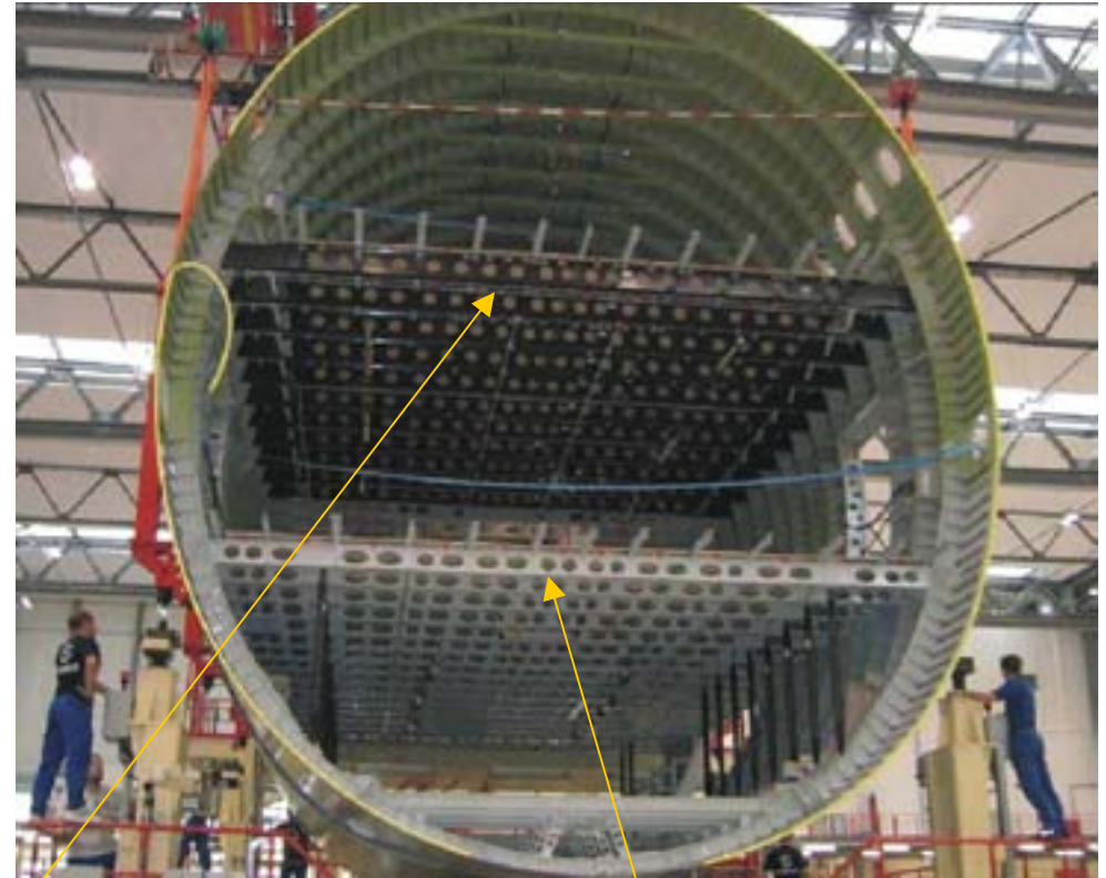
CFRP floor beams
