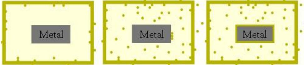
1. Sublimation (evaporation) of the VCI molecules from the carrier material
